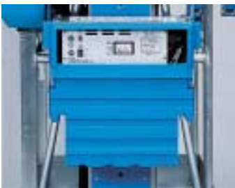
Removable battery box features separate compartments for the battery and charger.
